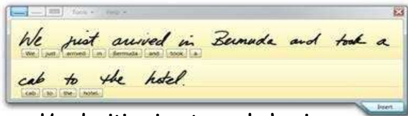
Handwriting input panel showing writing and recognized text
